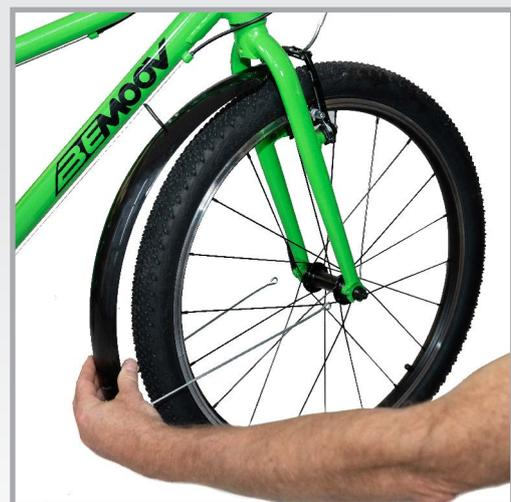
**Step 2.** Slide the front mudguard, with its black bracket, from the rear towards the front of the bike, under the fork and under the front brake cable. The black mounting bracket is positioned against the hole at the rear of the fork.
