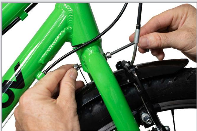
**Step 3.** Slide the screw A x1 into the fork hole from the front to the back of the bike, taking care to position the washer between the allen bit and the paint. Secure the mudguard in the lowest position by tightening the self-locking nut at the black mounting bracket.
